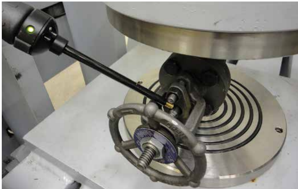
Pressurized with helium, this forged steel gate valve is being monitored for leakage through the stuffing box. The pictured emissions tester (wand with green light) can detect emissions as low as 5 \times 10^{-8} mbar l/s.
