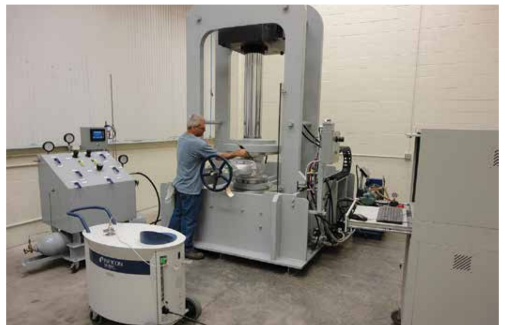
Low Emissions testing being performed in-house on Bonney Forge Eco-Seal® packed cast steel valves.
