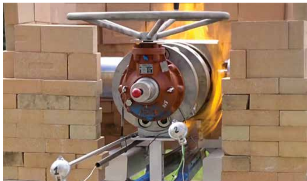
API 6FA fire testing being performed on made to order valve, this test ensures valves will perform in emergency situations.
