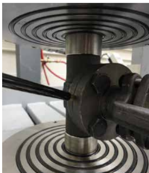
Same valve as above, is also subjected to emissions testing at the body/bonnet gasket area, similar to the requirements of ISO 15848-1.
